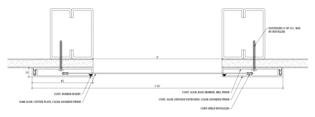
NOTE: 1 HOUR CONSTRUCTION INDICATED 2 LAYERS OF GYPSUM BOARD FOR 2 HOUR CONSTRUCTION
